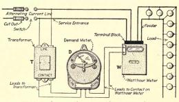
Fig. 22.—Method of connecting alternating-current demand meter for 440 and 660-volt loads. For 110 and 220-volt loads, and for direct-current loads the transformer is omitted.
